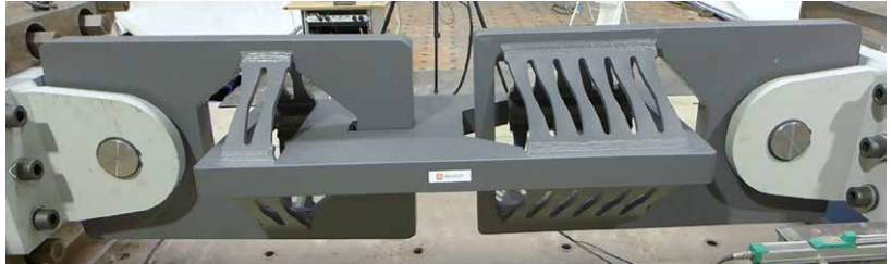
SHARK®-Adaptive at max compression displacement
