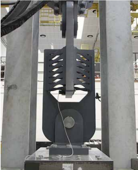
SHARK® at max tension position
