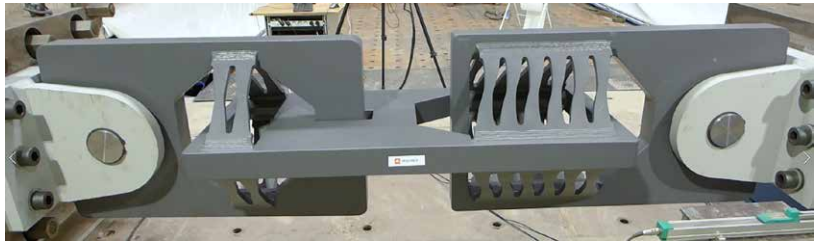
SHARK®-Adaptive at max tension displacement
