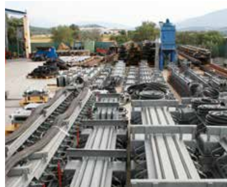
Different types of roadway expansion joints before shipment
