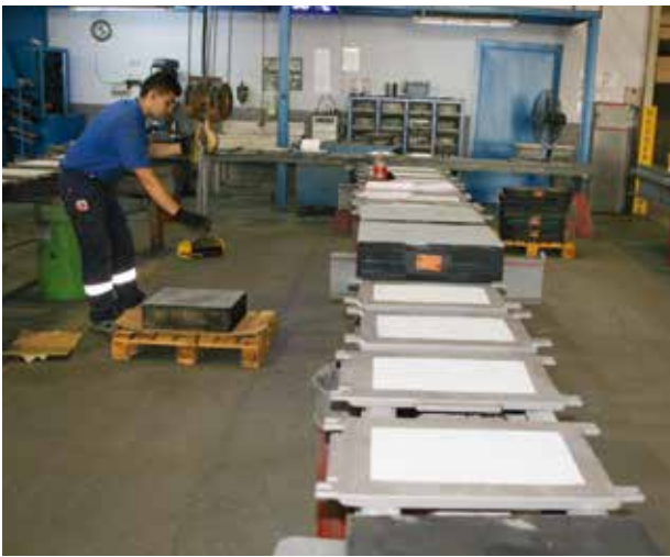
Elastomeric bearings during assembly
